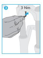
MONTAGE VORDERRADSCHUTZ · MOUNTING THE FRONT MUDGUARD
