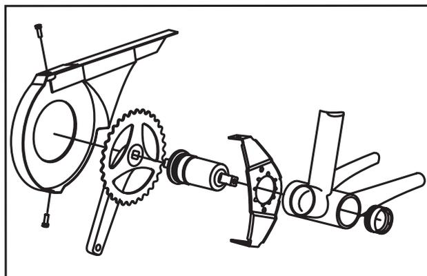
For installation crank and bottom bracket have to be disassembled. Special tooling equipment required. Please contact your dealer.
