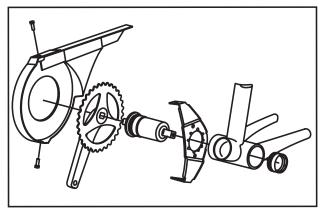
For installation crank and botton bracket have to be disassembled. Special tooling equipment required. Please contact your dealer.
