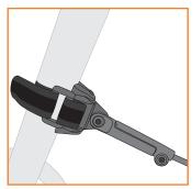
KEEP THE MINIMUM DISTANCE OF 15 MM BETWEEN FENDER AND TYRE.
