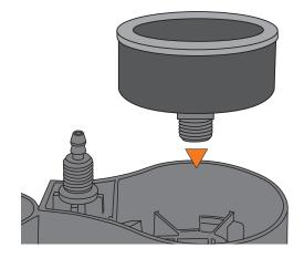
6. Push the pressure gauge cap down again and secure it with the union nut.
