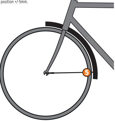
The lowest stay is to be mounted 25-65mm from the end of the mudguard (measured without the spoiler/edge protector)
