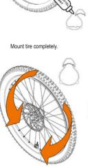
Preinstal the tyre and add sealant.
