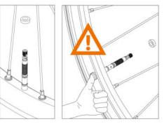
Hold the valve and attach the sensor housing. Serial number points to the wheel hub. Lightly lubricate the O-rings if necessary.
