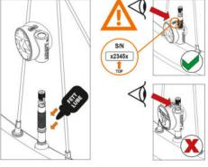
Hold the valve and put on the 2nd seal.
