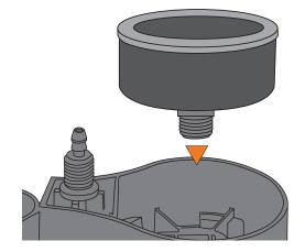
6. Push the pressure gauge cap down again and secure it with the union nut.
