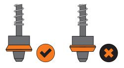
4. Grease the rubber cup seal, re-insert the cylinder rod and screw it in.
