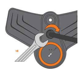
3. Unscrew the pressure gauge at the bottom with an Allen key (size 10).
