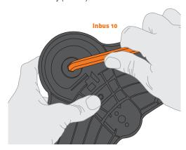
4. Turn the pressure gauge holder approximately 45° anti-clockwise until you feel resistance. Then pull out the pressure gauge holder.
