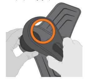
Turn the pressure gauge holder approximately 45° anti-clockwise until you feel resistance. Then pull out the pressure gauge holder.
