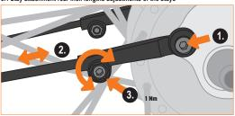
Mounting of spacers for frames with disc brakes
