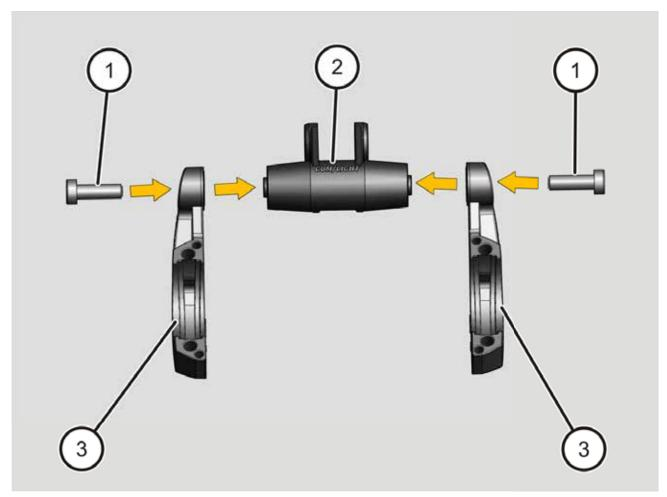
(i) The optional COM/CAM adapter can be mounted using the clamping arms analogue to the COM/LIGHT.
