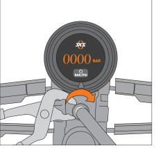
10. Tighten the hose screw connection again
