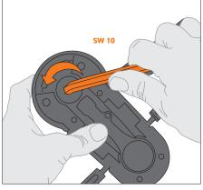
5. Unscrew the pressure gauge at the bottom with an Allen key (10)
