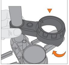
8. Put the pressure gauge cap back in place
