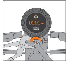
3. Loosen the hose screw connection
