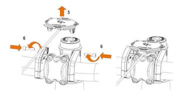
2. Connect the COMPIT to the e-bike For e-bikes with a 12 V-36 V lighting system or power supply
