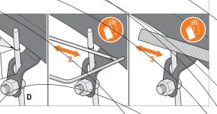
09 Tighten all screws on the struts (D) and on the sliding bridge (C).
