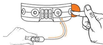
It is recommended to hold the cable while retracting it for a safer use.
