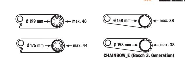
For installation crank and botton bracket have to be disassembled. Special tooling equipment required. Please contact your dealer.
