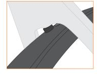
3.3.2 Screw the fender on the frame
