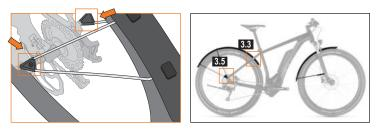
3.5.1 Stay attachment rear incl. lengths adjustments of the stays
